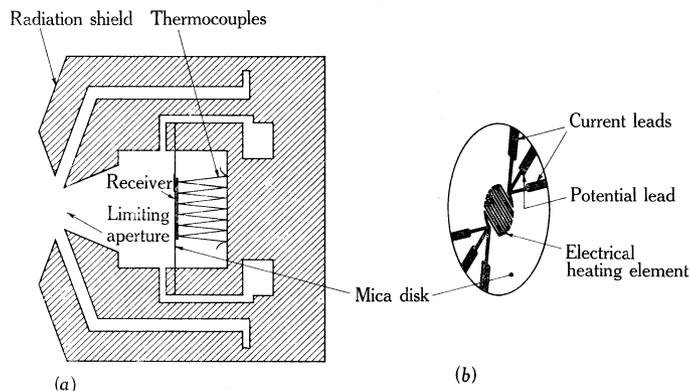
Fig. 4.—Schematic diagram of a Gillham-type absolute thermopile showing (a) the complete instrument in section and (b) the electrical heating element of evaporated gold on mica. Assembly details are similar to those described by Gillham (1962).
