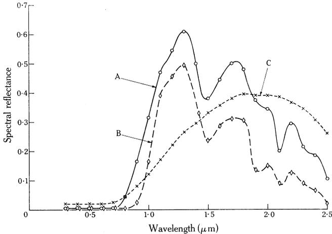
Fig. 3.—Curves of spectral reflectance for two black velvet cloths (curves A and B) from different sources and one black Italian cloth (curve C).
