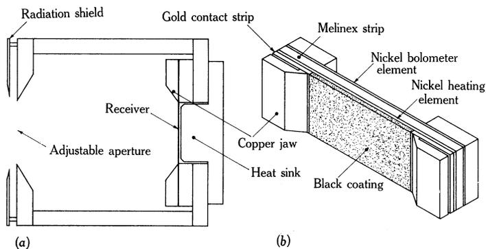
Fig. 5.—Schematic diagram of an absolute bolometer showing (a) the complete instrument in horizontal section and (b) the receiver drawn to a larger scale, with the thickness of the thin components greatly exaggerated.
