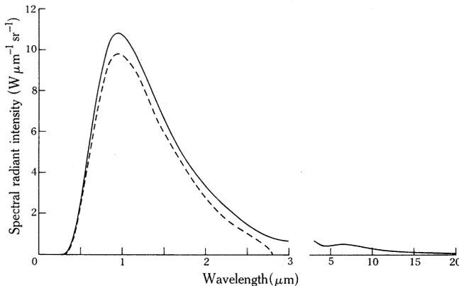
Fig. 2.—Curves of spectral radiant intensity for the lamp used as radiation source without a filter (full curve) and with a 14 mm thick filter of hard crown glass (dashed curve).
