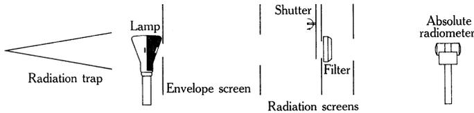
Fig. 1.—Experimental arrangement for absolute measurements of irradiance.
