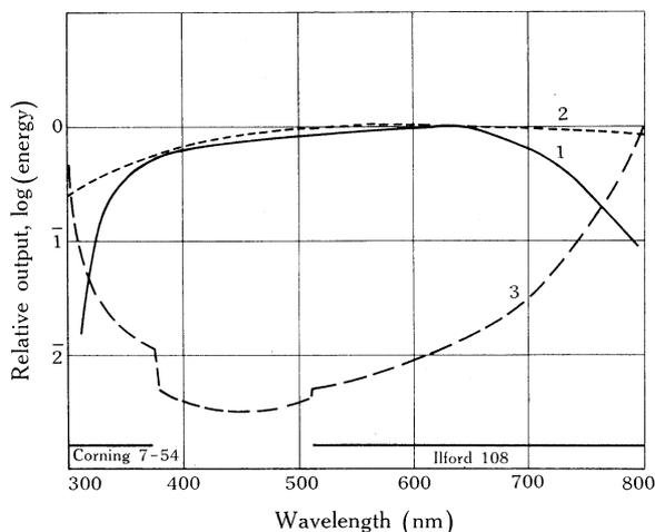
Fig. 3.—Chemiluminescent cloud output at night (curve 1, mean of 21 records). Also shown are the spectral distribution for black-body radiation at 5000°K (curve 2) and the photomultiplier dark current equivalent for the highest recorded intensity (curve 3).
