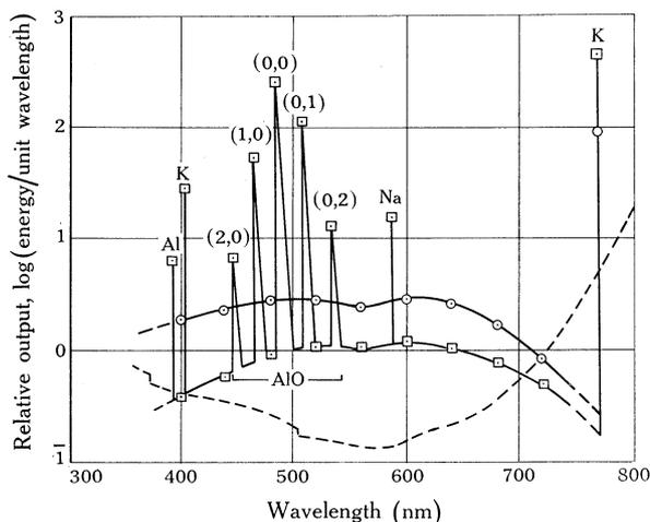
Fig. 4.—Chemiluminescent cloud outputs at twilight for two K-type glow clouds (○, dark, 125 km; □, sunlit, 148 km). The dashed curve shows the sky-dark current equivalent.
