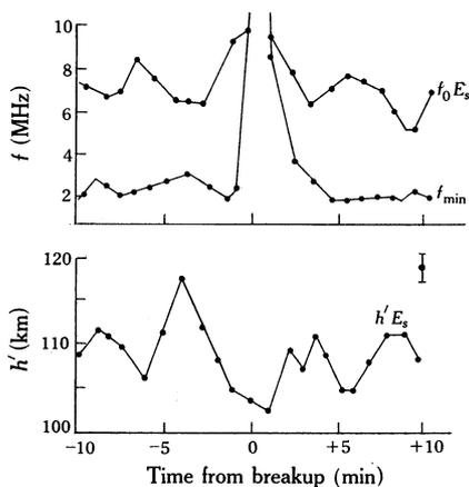
Fig. 1.—Patterns of behaviour of  $f_0E_s$ ,  $f_{min}$ , and  $h'E_s$  within  $\pm 10$  min of the breakup time.
