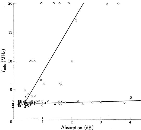
Fig. 3.—Scatter plot of ionosonde  $f_{\min}$  against riometer absorption data for the 10 min before and after breakup for the July sequences:
