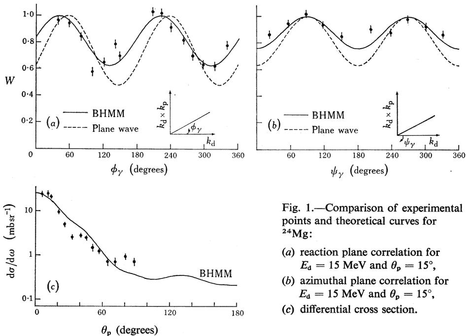
Fig. 1.—Comparison of experimental points and theoretical curves for  $^{24}\text{Mg}$ :
