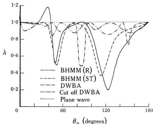
Fig. 5.—Angular dependence of the parameter  $\lambda = -2A_2^2/A_2^0$  for the  $^{44}\text{Ca}(d, p)$  reaction with  $E_d = 7.01$  MeV. The optical parameter sets R and ST used in the BHMM calculations are defined in Table 1.
