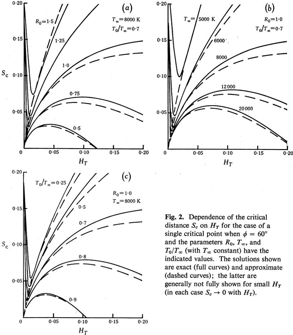
Fig. 2. Dependence of the critical distance  $S_c$  on  $H_T$  for the case of a single critical point when  $\phi = 60^\circ$  and the parameters  $R_0$ ,  $T_\infty$ , and  $T_0/T_\infty$  (with  $T_\infty$  constant) have the indicated values. The solutions shown are exact (full curves) and approximate (dashed curves); the latter are generally not fully shown for small  $H_T$  (in each case  $S_c \rightarrow 0$  with  $H_T$ ).
