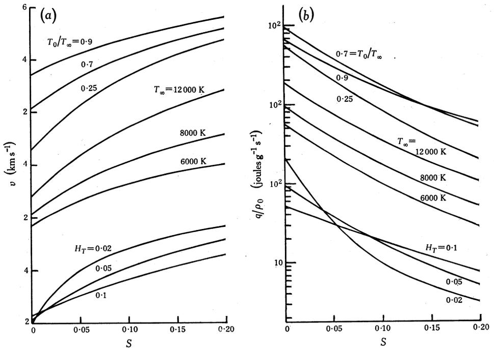
Fig. 3. Effect of variations in the parameters  $T_0/T_\infty$  (with  $T_\infty$  constant),  $T_\infty$  and  $H_T$  on the (a) velocity and (b) heating profiles for the case of a single critical point when  $\phi = 60^\circ$  and  $R_0 = 1$ . While each parameter is varied, the other two assume constant values appropriately from  $T_0/T_\infty = 0.7$ ,  $T_\infty = 8000$  K or  $H_T = 0.05$ . In (b) the specific heat ratio  $\gamma$  is taken to be 1.67.
