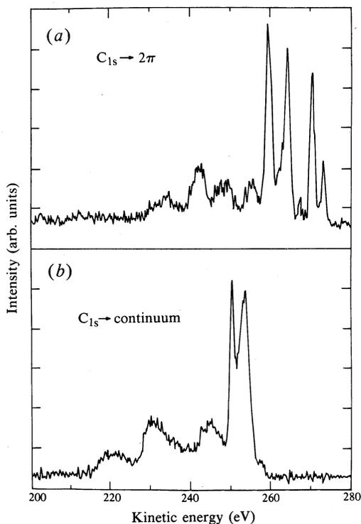
**Fig. 4.** Electron energy distribution curves of the electrons created in the decay of the primary  $C_{1s}$  core hole excited state in CO. In (a) the decay of the  $C_{1s} \rightarrow 2\pi$  excitation is shown, while (b) shows the 'standard' Auger spectrum following  $C_{1s}$  ionisation.
