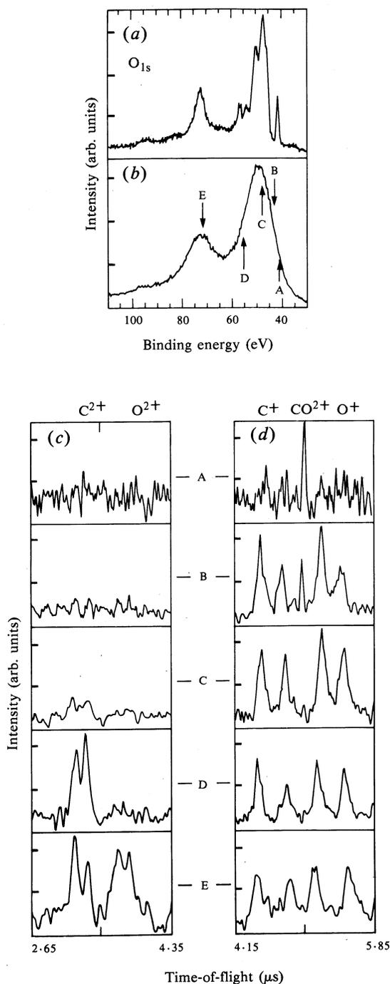
**Fig. 7.** The TOF ion mass spectra of CO taken in coincidence with oxygen Auger electrons of various kinetic energies as indicated by the arrows A-E in the Auger spectrum (b). A comparison is shown of the Auger spectra taken without (a) and with (b) an ion extractor field applied across the ionisation region. The TOF mass spectra (c) show the region where  $C^{2+}$  and  $O^{2+}$  are expected to arrive and spectra (d) show the region containing  $C^+$ ,  $CO^{2+}$  and  $O^+$ .
