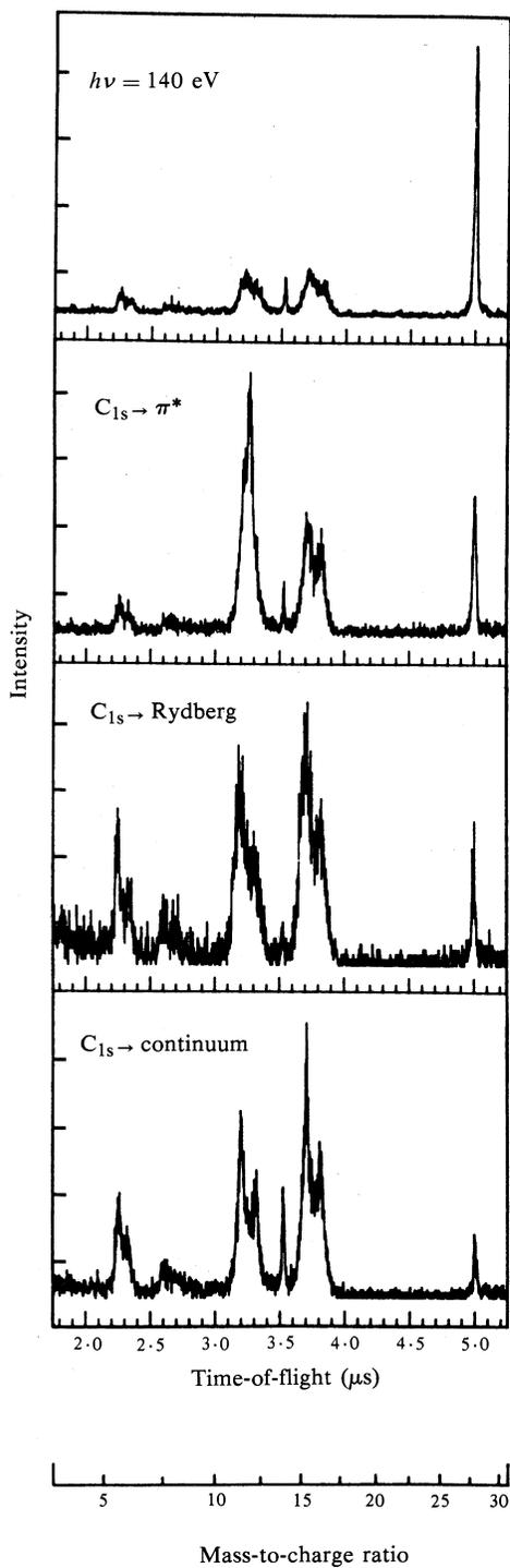
**Fig. 2.** The CO fragment ion mass spectra measured with a TOF mass spectrometer. The spectra are taken at different excitation energies to reflect the effect of the primary excitation on the branching ratio of the ionic fragments.
