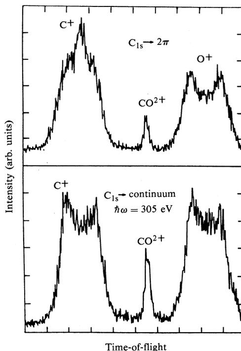
**Fig. 3.** High resolution mass spectrometer scan from  $m/e = 12-16$ . The sharp peak in the centre is due to  $CO^{2+}$  having only thermal energy. The other peaks show substructure and substantial broadening due to the kinetic energy distribution of the fragments.
