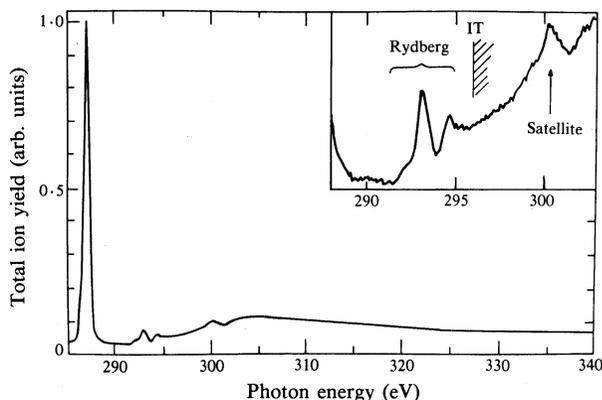
**Fig. 1.** Total ion yield of CO near the onset of the  $C_{1s}$  excitation. The total ion yield closely resembles the absorption and shows structures due to  $C_{1s}$  transitions into various types of final states.
