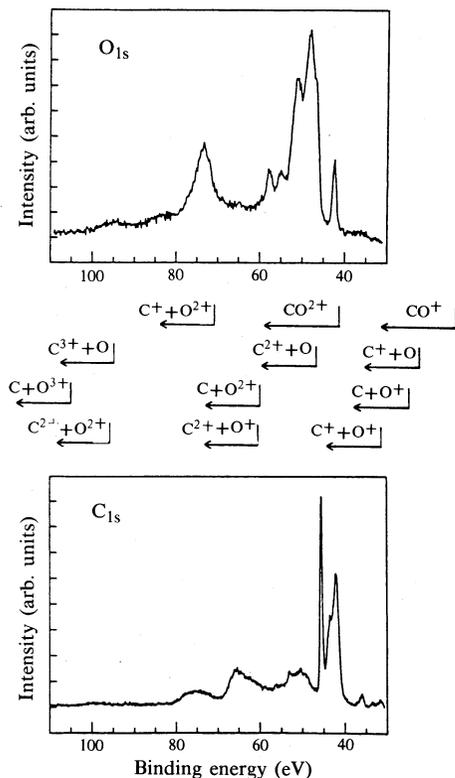
**Fig. 5.** The CO oxygen and carbon Auger spectra and adiabatic energy thresholds for the production of various ionic fragments. An Auger electron and the corresponding double hole configuration that is found to the right of any one of the thresholds cannot be associated with that particular fragmentation channel because it has carried too much energy out of the system.
