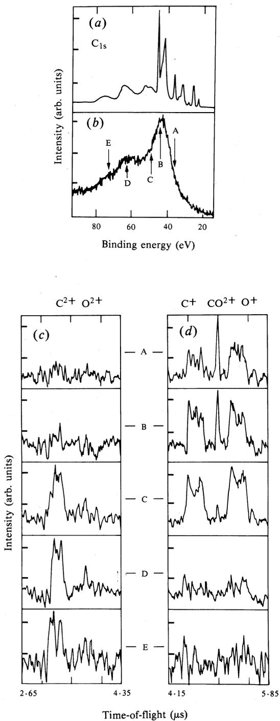
Fig. 8. The TOF ion mass spectra of CO taken in coincidence with carbon Auger electrons (see Fig. 7 for details).
