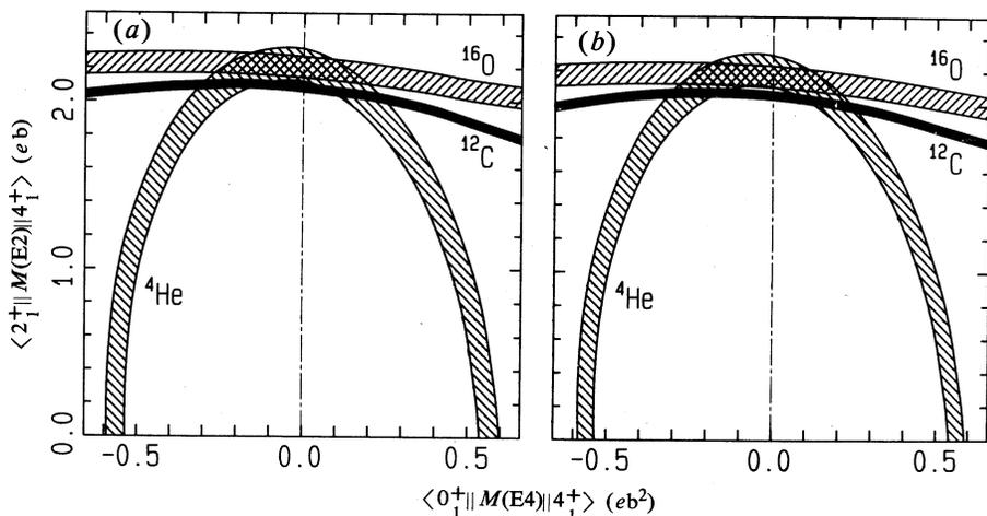
Fig. 2. Loci of values of  $\langle 0_1^+ \| M(E4) \| 4_1^+ \rangle$  and  $\langle 2_1^+ \| M(E2) \| 4_1^+ \rangle$  consistent with the measured excitation probabilities of the  $4_1^+$  state of  $^{194}\text{Pt}$  under  $^4\text{He}$ ,  $^{12}\text{C}$  and  $^{16}\text{O}$  bombardment assuming  $\langle 2_2^+ \| M(E2) \| 4_1^+ \rangle = 0$ , and (a)  $Q(4_1^+) = 0$  and (b)  $Q(4_1^+) = 0.8 eb$ .
