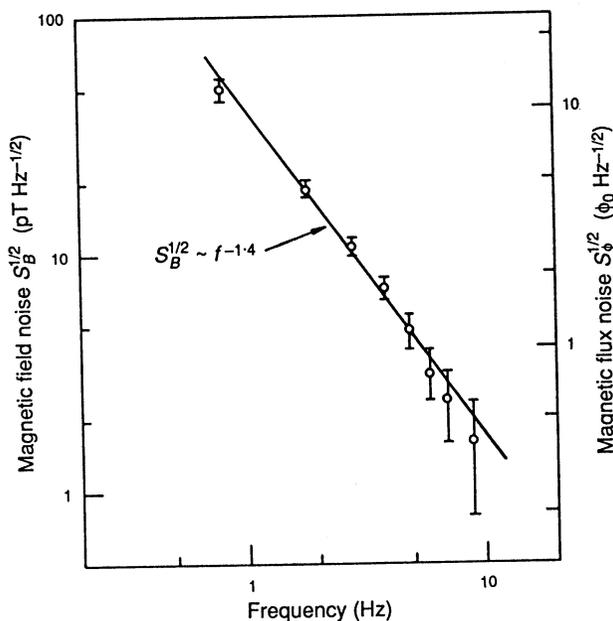
Fig. 2. Measured low-frequency noise in YBCO.
