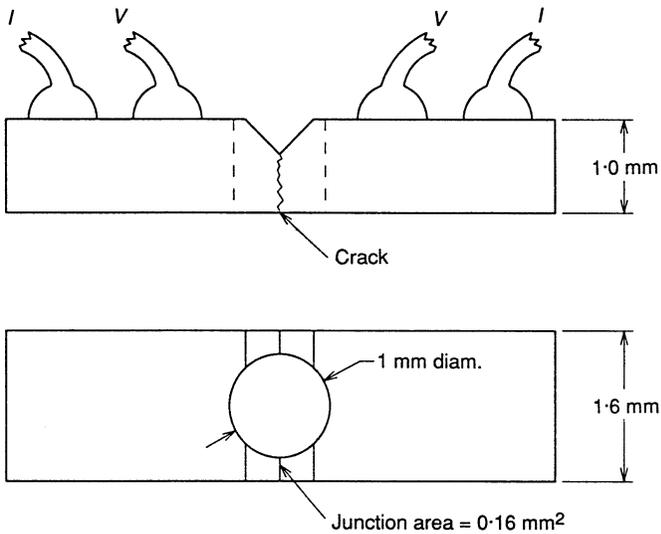
**Fig. 3.** Design for break-junction YBCO d.c. SQUID.
