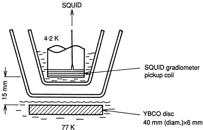
**Fig. 1.** Apparatus for measurement of YBCO flux noise.
