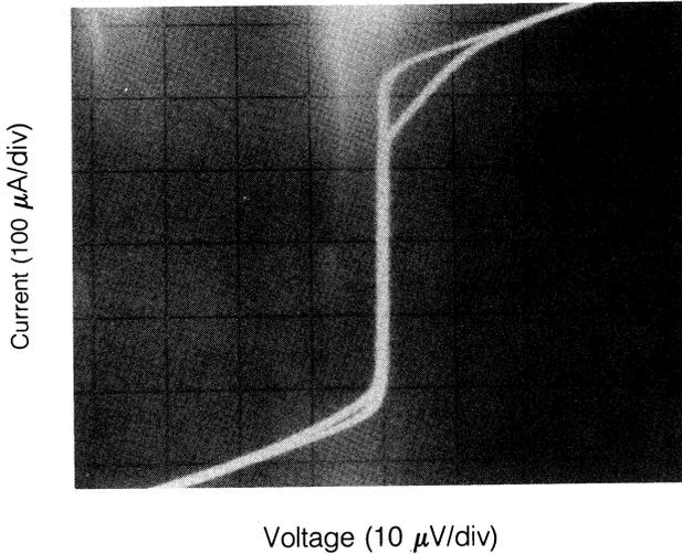
**Fig. 4.** SQUID current-voltage characteristics.
