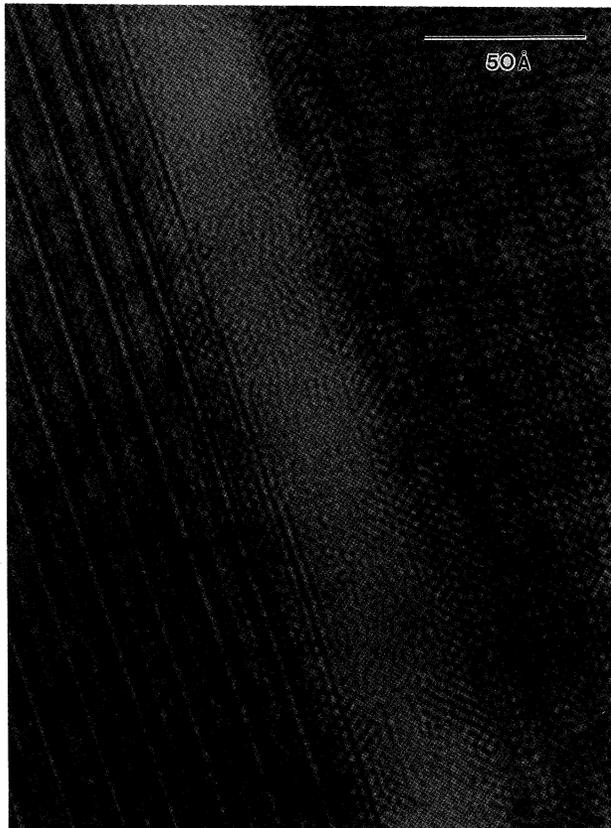
**Fig. 7.** Intercalation of an amorphous region in a monocystal.
