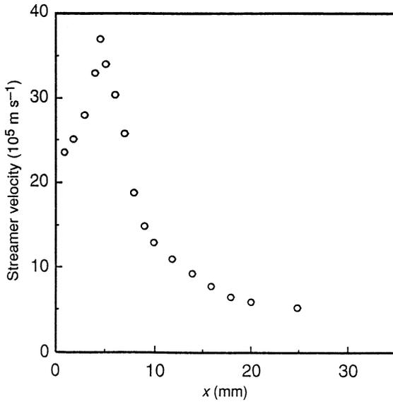
**Fig. 4.** Measured streamer velocity versus position in air, for a 35 mm gap with 25 kV applied (reproduced from Creighton *et al.* 1992).
