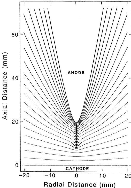
**Fig. 1.** Equipotential contours, at 1 kV intervals, for a 20 mm gap in air with 20 kV applied, showing the streamer development after 12.5 ns.
