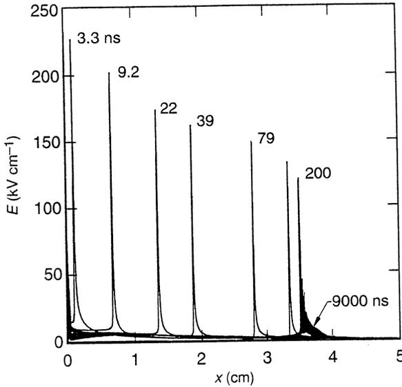
Fig. 5. Electric field distributions at various times in ns, for a 55 mm gap in air with 20 kV applied.
