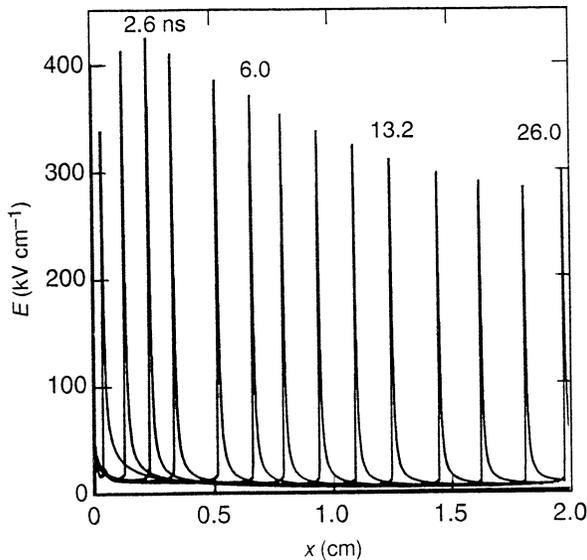
**Fig. 2.** Electric field distributions computed along the centre line of the potential distributions of the type shown in Fig. 1, at various times shown in ns.
