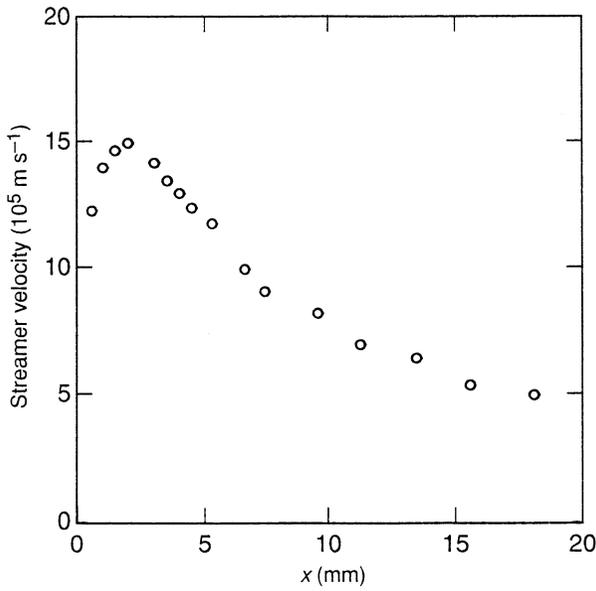
**Fig. 3.** Computed streamer velocity versus position in air, for a 20 mm gap with 20 kV applied.
