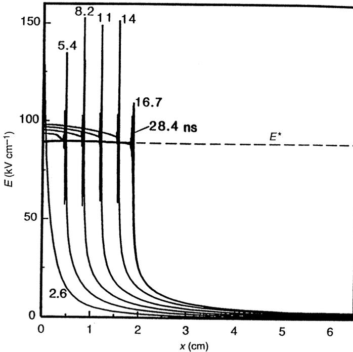
**Fig. 6.** Electric field distributions at various times in ns, for a 65 mm gap in SF<sub>6</sub>, with 200 kV applied.
