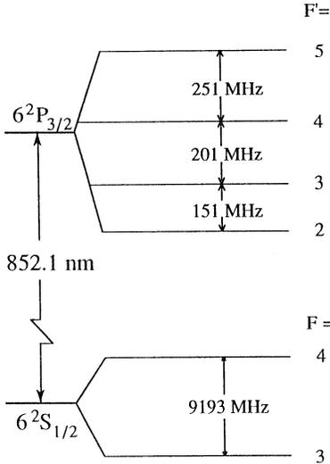
**Fig. 1.** Energy level diagram for the  $6^2S_{1/2}$ - $6^2P_{3/2}$  transition of  $^{133}\text{Cs}$ .
