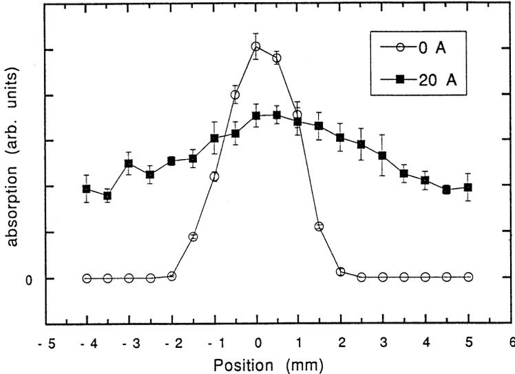
**Fig. 6.** Spatial distribution of atoms after moving past a wire carrying 0 A and 20 A. The 20 A curve has an exaggerated vertical scale; the area beneath the two curves should be equal. The origin of the horizontal axis is defined by the centre of the undeflected (0 A) distribution. Negative positions indicate deflection away from the wire, positive positions indicate deflection toward the wire.
