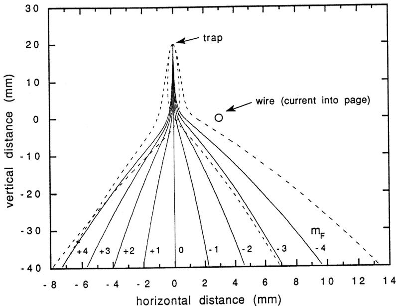
**Fig. 7.** Computer simulation of trajectories of atoms deflected by the magnetic field from a wire carrying 20 A. The solid lines indicate the trajectories for atoms in the nine possible magnetic substates, assuming zero initial velocity. The broken lines are for atoms in the  $m_F = \pm F$  substates with initial transverse velocities of  $\pm 1 \text{ cm s}^{-1}$ , showing the converging (diverging) nature of the deflection for atoms in repulsive (attractive) substates.
