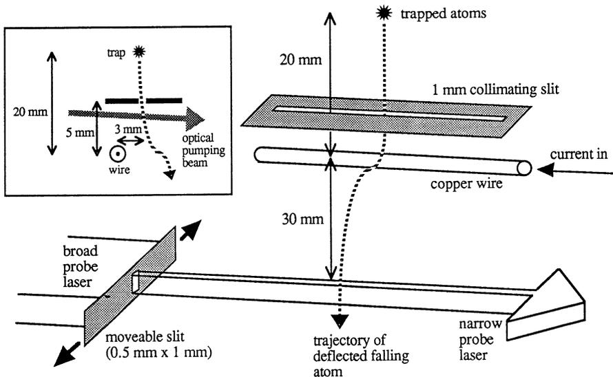
**Fig. 5.** Apparatus for deflecting slowly-moving atoms with the magnetic field from a current-carrying wire. Inset shows view end-on to the wire, indicating the position of the optical pumping laser beam.
