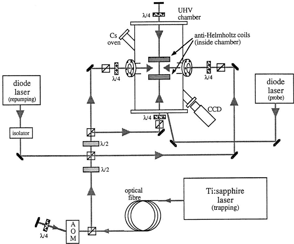
**Fig. 2.** Schematic diagram of the experimental layout for laser trapping and cooling of caesium atoms. The two laser beams that are drawn as entering the vacuum chamber horizontally actually enter at  $45^\circ$  to the plane of the page, and are retroreflected by mirrors beneath the chamber. AOM: acousto-optic modulator, CCD: charge-coupled-device camera,  $\lambda/2$ : half-wave plates, and  $\lambda/4$ : quarter-wave plates.
