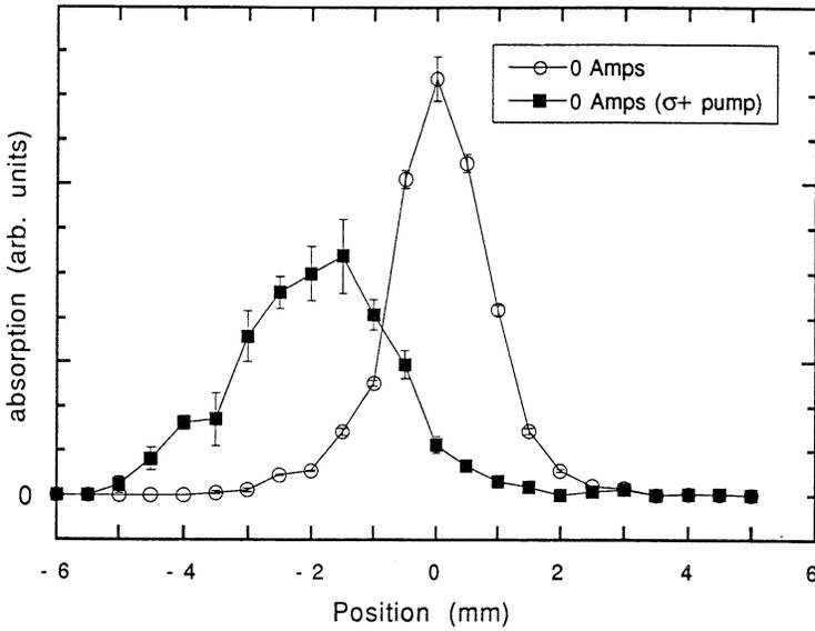
**Fig. 8.** Spatial distribution of falling atoms with and without optical pumping beam, with no current through the wire. The optical deflection is independent of the polarisation of the optical pumping radiation. The deflected distribution is broadened by the randomly directed momentum transferred to the atoms by each absorption/spontaneous emission cycle.
