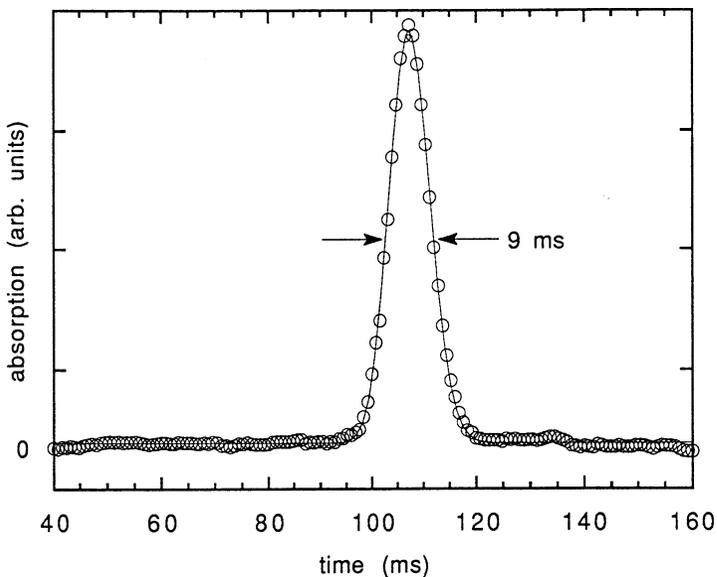
**Fig. 4.** Absorption signal from time-of-flight measurement. The circles are the experimental points; the solid line is a fitted curve giving a temperature of  $22 \mu\text{K}$ . Horizontal axis is the time elapsed since the atoms are released from the trap.
