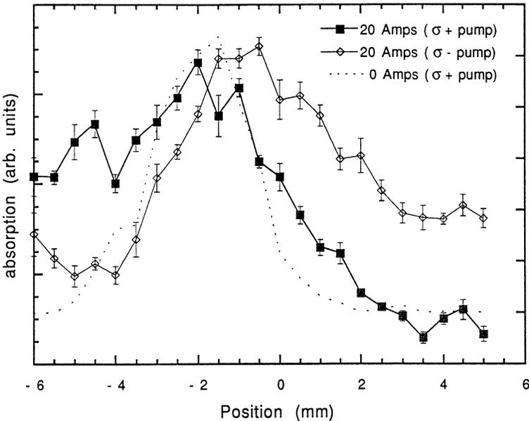
**Fig. 9.** Spatial distribution of optically pumped atoms falling past a wire carrying 20 A. Each sense of circular polarisation of the optical pumping radiation (given by  $\pm 45^\circ$  rotation of quarter-wave plate) gives enhanced deflection to one side of the wire. The optically-pumped 0 A distribution is included to show the effect of optical deflection.
