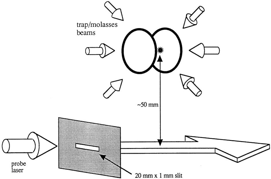
**Fig. 3.** Time-of-flight measurement of falling atoms by absorption of a 'ribbon' of resonant laser light.
