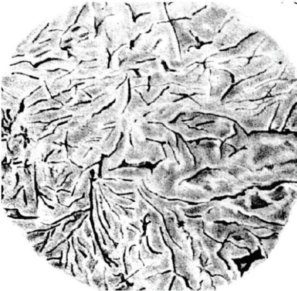
Figure 1: Optical micrograph of a section of a mould made of gray iron (Martens 1878) copied from Portella (2006).
