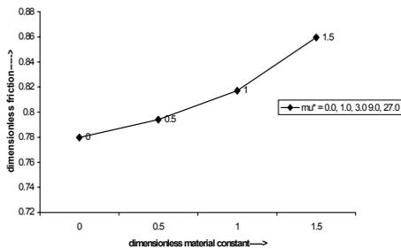
**Figure 3.** Dimensionless friction  $\bar{F}$  for different values of dimensionless magnetization parameter  $\mu^*$  ( $\mu^*$ ) and dimensionless material constant  $\beta^2$ .
