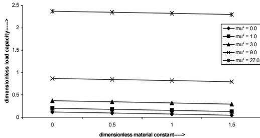
**Figure 2.** Dimensionless load capacity  $\bar{W}$  for different values of dimensionless magnetization parameter  $\mu^*$  ( $\mu^*$ ) and dimensionless material constant  $\beta^2$ .
