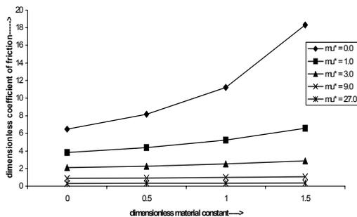
**Figure 4.** Dimensionless coefficient of friction  $\bar{f}$  for different values of dimensionless magnetization parameter  $\mu^*$  ( $\mu^*$ ) and dimensionless material constant  $\beta^2$ .
