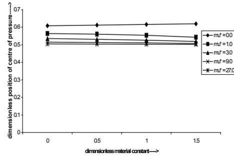
**Figure 5.** Dimensionless position of centre of pressure  $\bar{Y}$  for different values of dimensionless magnetization parameter  $\mu^*$  ( $\mu^*$ ) and dimensionless material constant  $\beta^2$ .
