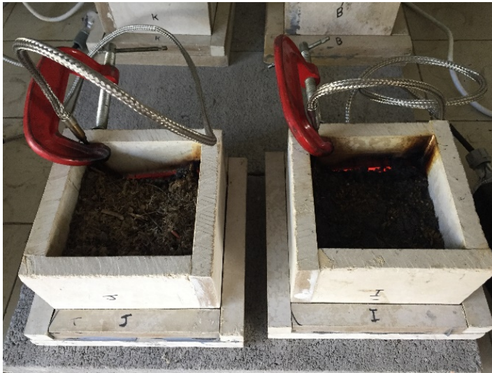
Fig. S3. Custom-built burn boxes (10 x 10 x 7 cm), with soil Block B inside and coil heater inserted, held in place with a G-clamp.
