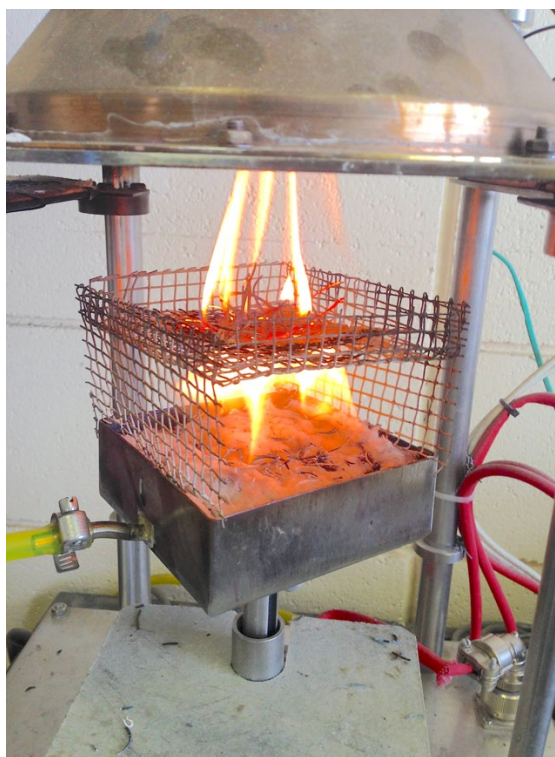
Fig. S1. Modified setup for the cone calorimeter flammability testing.
