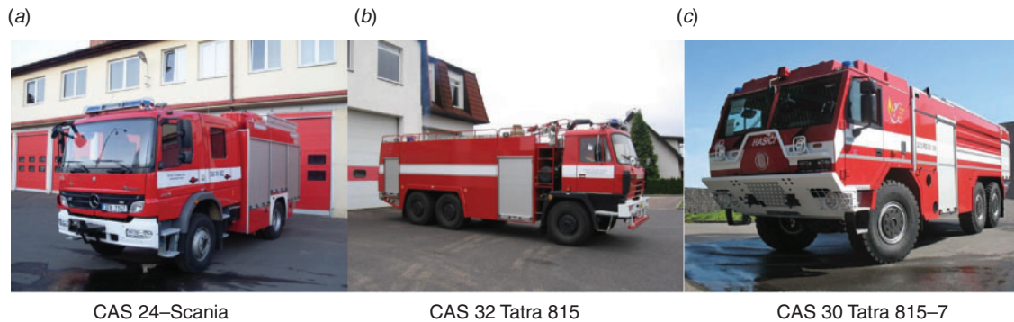
Fig. 3. Firefighting vehicles commonly used by Fire Rescue Service of the Czech Republic: (a) road; (b) mixed; and (c) off-road.
