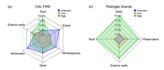
**Fig. 4.** (a) Distribution of low fire protection (red), high fire protection (green), and unknown (blue) building features considered in the CAL FIRE database and (b) in the Pedrógão Grande database.
