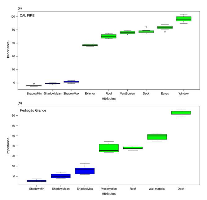
Fig. 7. Importance of independent variables in (a) CAL FIRE database and (b) Pedrógão Grande database calculated by Boruta feature selection.
