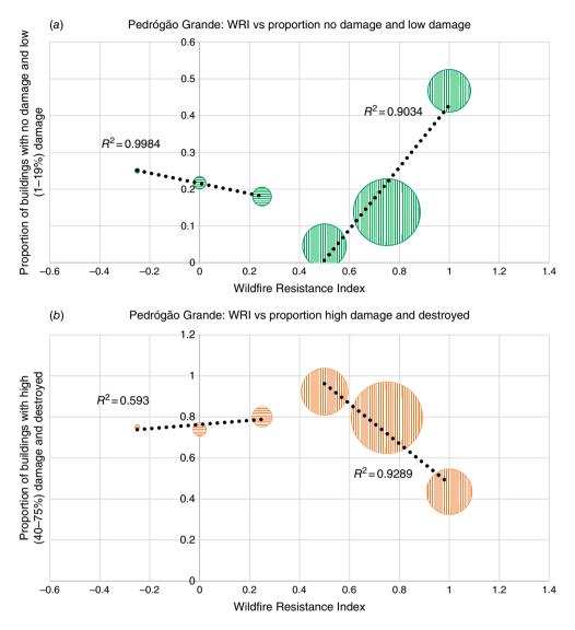
**Fig. 10.** Pedrógão Grande data: WRI against proportion of buildings with (a) no damage or low (1–19%) damage after wildfire and (b) high (40–75%) damage and were destroyed after wildfire. The size of the circles plotted is proportional to the number of buildings in each WRI value.
