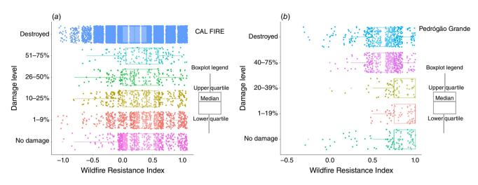
Fig. 8. WRI and damage level distribution and relationship with boxplot and jitter plot in (a) CAL FIRE database and (b) Pedrógão Grande database.
