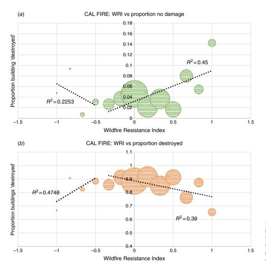
**Fig. 9.** CAL FIRE data: WRI against proportion of buildings that (*a*) experienced no damage and (*b*) were destroyed after wildfire. The size of the circles plotted is proportional to the number of buildings in each WRI value.
