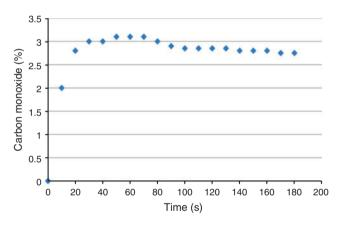
**Fig. 2.** Concentration of carbon monoxide (%CO) in cooled exhaust from a 25-cc petrol engine without a catalytic converter (four-stroke whippersnipper) from a cold start. In a petrol engine without a catalytic converter, CO concentration rises initially and then reaches a plateau at a relatively high concentration.
