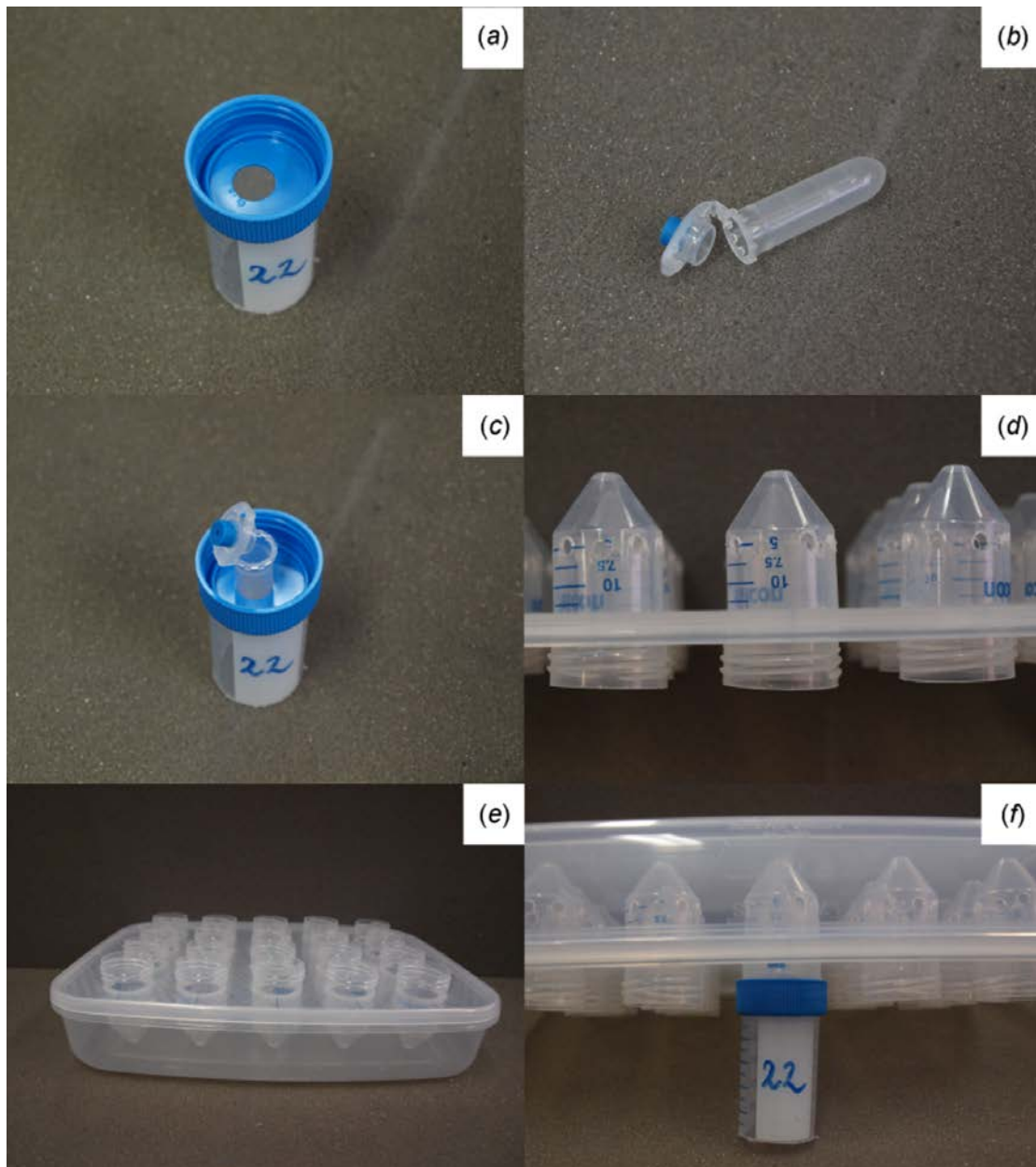
Fig. S1. Close-up views of the custom-made transpiration chamber: (a) Socket for the Eppendorf tubes; (b) Eppendorf tube with rubber seal; (c) Assembled berry holder unit; (d) Lid of the transpiration chamber with individual berry cells; (e) Complete transpiration chamber (upside down); (f) Transpiration chamber with one berry holder unit attached.
