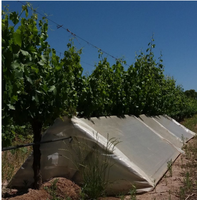
Fig. S1. Heating system consisting of an open-top chamber installed under 5 consecutive vines along the row to increase air temperature during 2016/17 and 2017/18 seasons. Heating systems were installed in five replicates of each variety (Grenache and Syrah). Mendoza.
